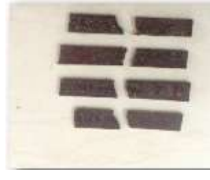
Figure 4.6 - Impact test specimen after test
